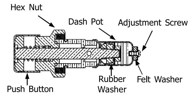
**To Install:** Remove old flush valve assembly and make sure the valve is free from debris or defects. Install flush valve into the assembly and tighten. Tighten to 90 in/lbs pressure.
